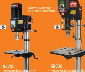
Powerful direct drive 1 HP high torque motor with no pulleys or belts Spindle taper MT #2 Comes with 5/8" drill chuck & key, firmware USB cable
